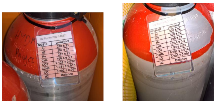
Figure 1. NPL reference materials supplied to ZSW and ZBT for evaluating analytical performance according to ISO/FDIS 14687 and EN 17124:2018.
